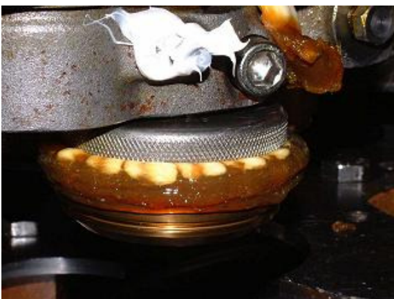
Seamer roll been lubricated with a food grade grease
