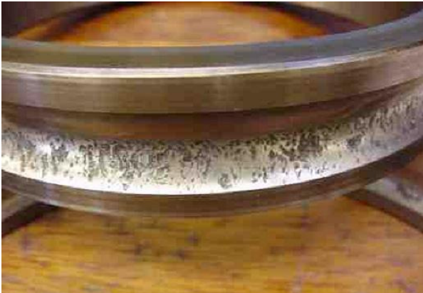
A failed axially loaded bearing from Angelus 121L can seamer (running on competitor oil) - shows heavy pitting, formed by contact staining after water ingress
