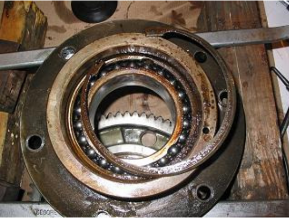
One of the main roller bearings of an Angelus can seamer been contaminated with sugar deposits
